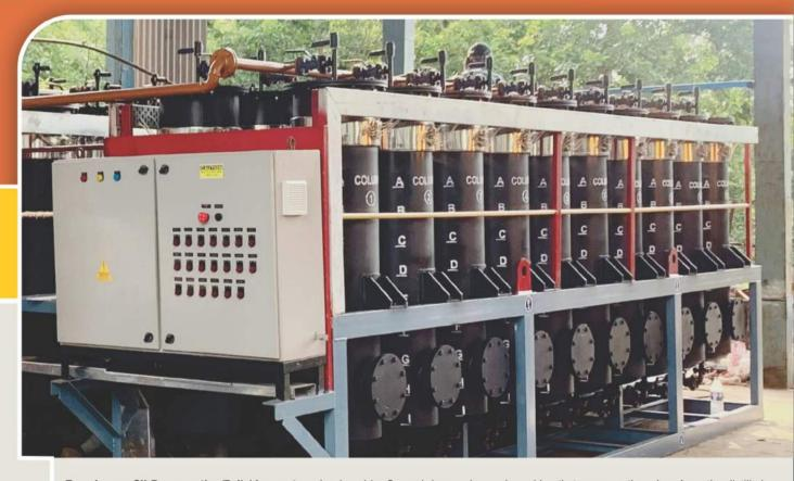
Transformer Oil Regeneration/Polishing system developed by Sumesh is an advanced machine that removes the odour from the distilled Transformer oil, apart from a drastic improvement in colour. This machine prevents industries from discarding the contaminated transformer oil, lube oil, hydraulic oil, turbine oil etc after removing the carbon content present in these oils after distillation process. This is an economical and an environmental friendly alternative to clay/hydrogen processing plant.
